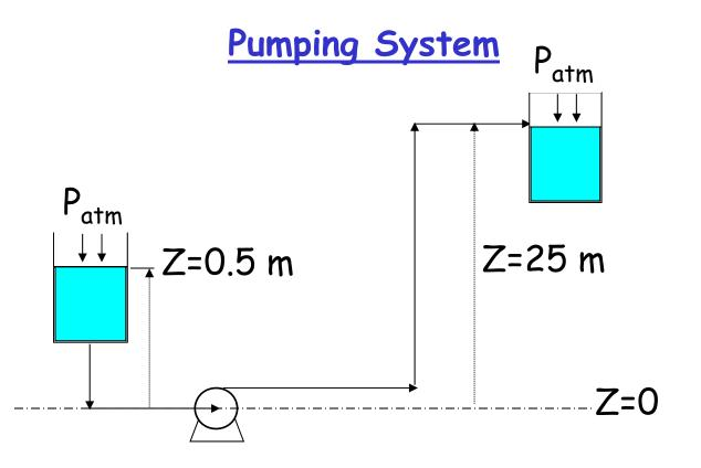
Suction line length (including fittings equivalent lengths) 12 Discharge line length (including fittings equivalent lengths) 50 ID of the suction pipe 0.4064 m, ID of the discharge line 0.3 Water flow at 0.75 m<sup>3</sup>/min.
